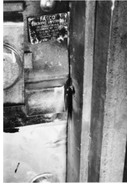
Cut through Bolt
